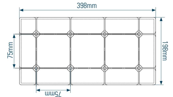
Drill holes suitable for M8 screws
